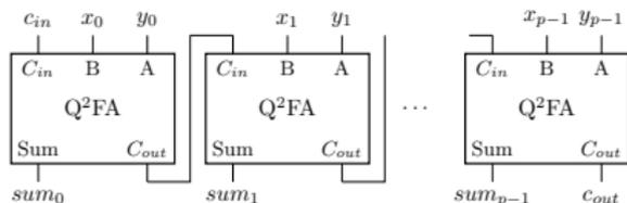
Fig 11: Schematic of quanternary quantum carry-ripple adder (Q<sup>2</sup>CRA)
