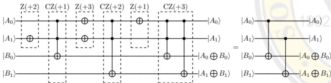
Fig 3: Common approach to quaternary CX and simplified operation
