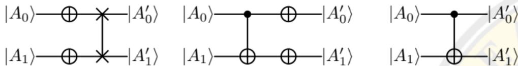
Fig 2: Z(03), Z(0321), and Z(23) Gates after Mapping
